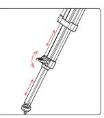
Flip Leg Lock Levers down and slide Leg sections to adjust height. Flip Levers up to lock.
