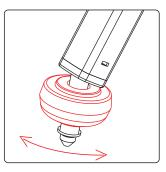
Rotate Rubber Foot clockwise to expose Spikes for outdoor use. Use Rubber Feet indoors.
