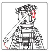
Loosen Pan Arm Locking Lever and raise Arm to comfortable position, then re-lock.
