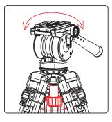
Loosen Head Lock Handle and pivot Head in Bowl of Tripod until it is level, then tighten.
