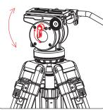
Tilt Drag/Lock lever provides both Drag and Locking control of vertical head movement.
