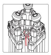
Pull Tab on circular Locking Clip, then spread Legs to full open position.
