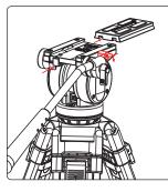
Loosen Quick Release Plate Lock Lever and press the QR Safety Button to allow QR Plate to be removed. Attach Plate to bottom of Camera using Mounting Screw then slide back on to Head. Slide and position for best balance and tighten QR Plate Lock Lever.
